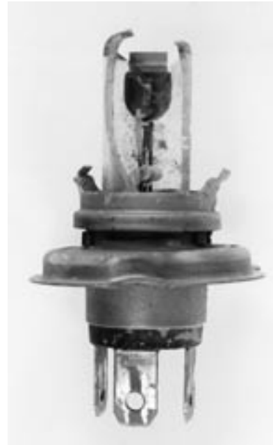
FIG. 2—H4 type bulb from the broken optical set, before the final cleaning with ultrasounds.
